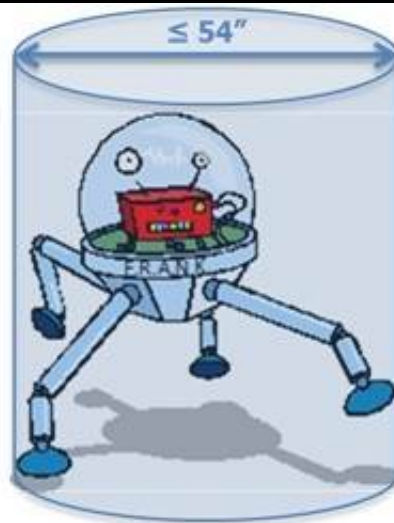
Figure 3-5a: ROBOT inside 54 in. diameter cylinder
